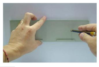
**Step 6** Prefer to drill a small hole on the location mark for easy mounting of the screws.
