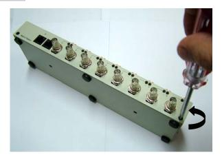
**Step 2** Hold onto the main case assembly with one hand supporting the top cover.
